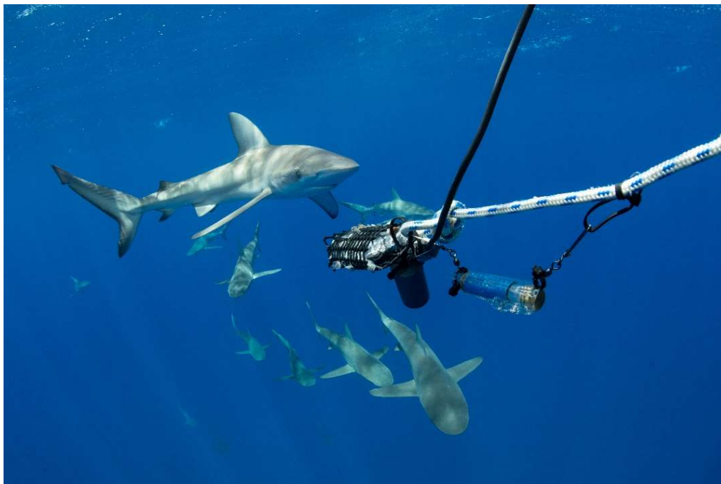
Scientific testing of shark deterrent devices in the Lord Howe Island Marine Park, showing active and inactive control devices mounted close to a bait bag. Photo credit DPIRD.
