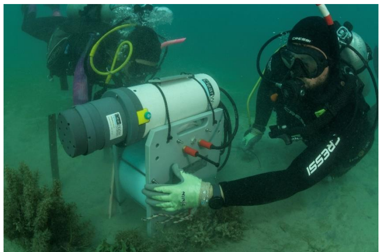
AIMS researchers sampling seawater (top) and deploying a nutrient sensor (bottom) in the LHIMP. Photo credit NSW DPI
